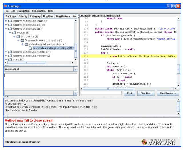
The upper left-hand pane of the window shows the bug tree; this is a hierarchical representation of all of the potential bugs detected in the analyzed Jar files.
